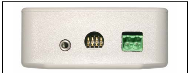
Figure 2: WME (Wood Moisture Equivalent) Terminal Block for Custom Probes and WME Socket for Protimeter plug in Probes. Channel 2 Shown for QuikStick, HygroStick and Surface Temperature Probe.
